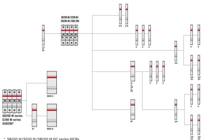
\* SB200 M/S200 M/SB200 M DC series MCBs and SDB200 switch disconnectors up to 3P or 2P+ST can be coupled with MOD-S
