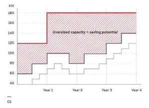
Standalone solution 2×60kW (N+1) UPS until year 1 3×60kW (N+1) UPS years 1-4 Oversized capacity Modular solution 20kW UPS modules can be added or removed at any time according to the actual need.
