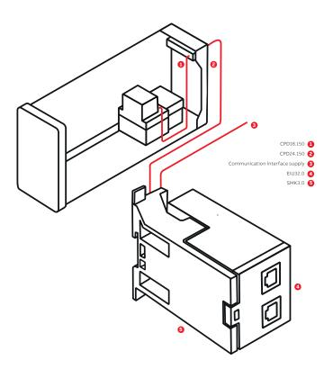
Separate wiring of the EtherNet/IP<sup>™</sup> communication interface EIU32.0
